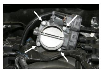
**4.** Install the provided bolts and washers thru the throttlebody and Poweraid Spacer and tighten to the manufacturer's specifications.
