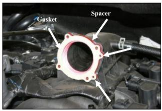
**3.** Install the Poweraid Spacer into the intake manifold as shown. Make sure the spacer is seated correctly over the two alignment pins on the intake manifold. Make sure the "flow" arrow printed on the spacer, points towards the intake manifold and away from the throttlebody. Next install the fiber gasket and the throttlebody.
