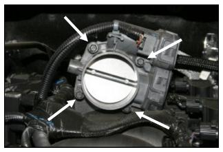
**2.** Remove the four bolts that secure the throttlebody to the intake manifold. Remove the throttlebody from the intake manifold and set it aside. (*No need to disconnect the wiring harness.*)
