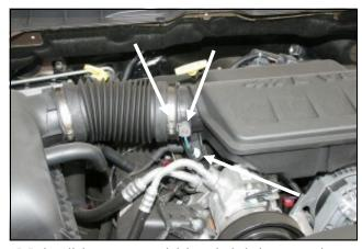
**5.** Reinstall the resonator and tighten the bolt that secures it to the intake manifold. Reinstall the intake tube, tighten the hose clamp, and reconnect the intake temperature sensor. **Re-connect the negative battery cable!**
